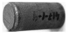
Fig. 5. Appearance of the core sample from Vyngapurovskoye oil and gas condensate field after dynamic and static tests on the FDES-645 unit
