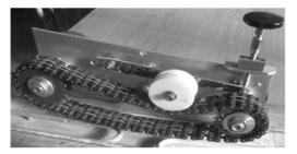
Fig. 6. Converter model with one working ring in the chain link
